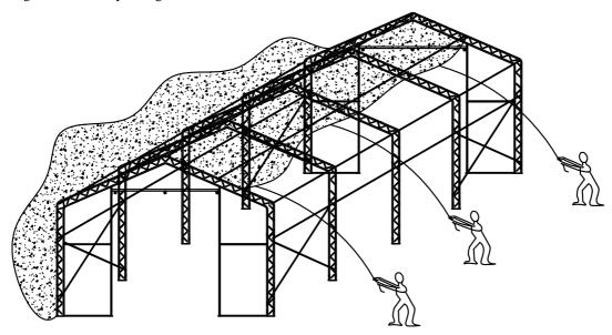
Figure 7 Pull the Roof Cover over the frame evenly
